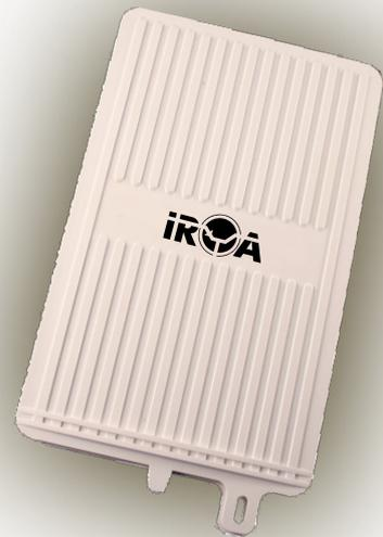
IPM 05 is microcontroller based prepaid energy meter which is especially designed for solar ac micro grids. It has 5 channels and each of them can be programmed separately for desired watt hour credit, watt limit and number of days .Multi channel design allows to connect 5 different households using a single meter but measuring usage of individuals at same time.
